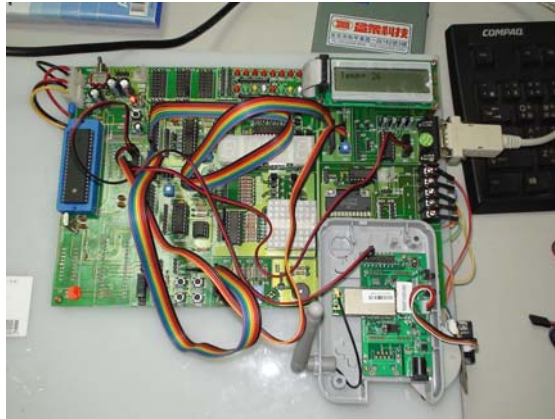
Figure 9 The implementation diagram of WSN for temperature monitor
