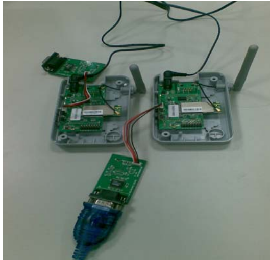
Figure 6 The development boards of WSN
