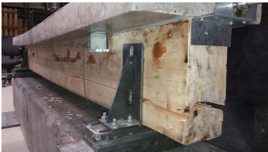
Figure 9 Shearing of the last lamella layer
