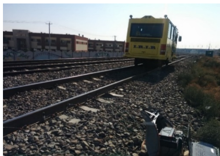
Figure 7 The drezin used for system calibration
