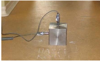
Figure 3 Sensors of acceleration above the main pivot
