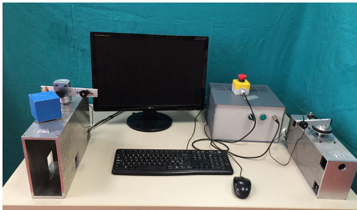
Figure 8 Bilateral teleoperation test bench.
