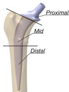
Figure 7 Geometrical segments of the femoral prosthesis body
