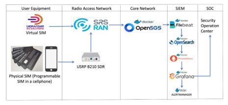
Figure 3 The high-level design of our 5F environment and SIEM
