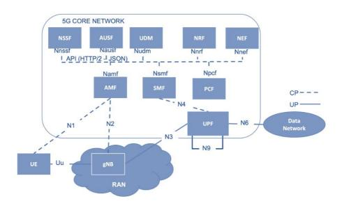
Figure 1 The architecure of 5G network
