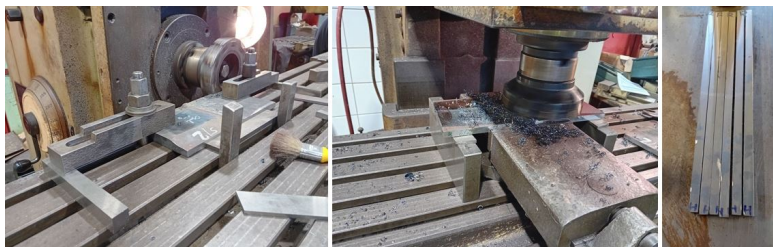
Figure 8 Milling and cutting of the plates for the laboratory tests
