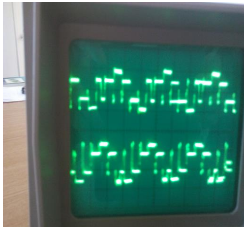
Figure 17 The output voltages - Phases U_R and U_S
