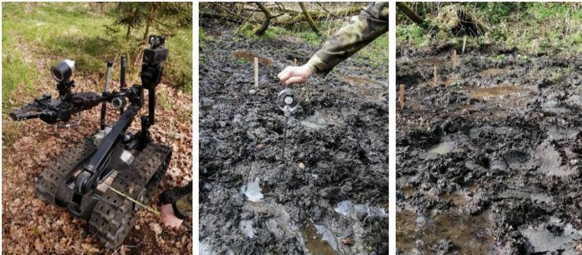
The marked low endurable terrain, measurement with cone penetrometer and measuring of the features of robotic device
