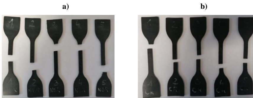
Figure 6 Test samples: (a) NBR; (b) CR
