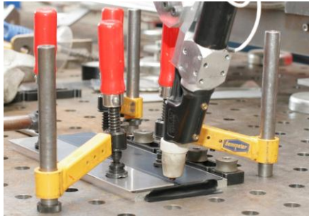
Figure 1 Plasma arc welding configuration
