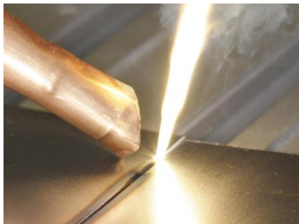
Figure 2 Solid-state laser beam welding process
