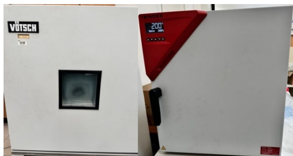
Figure 8 Vötsch and Binder climatic chambers for exact tempering of the specimens
