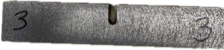
Figure 4 Charpy specimen with U shape notch
