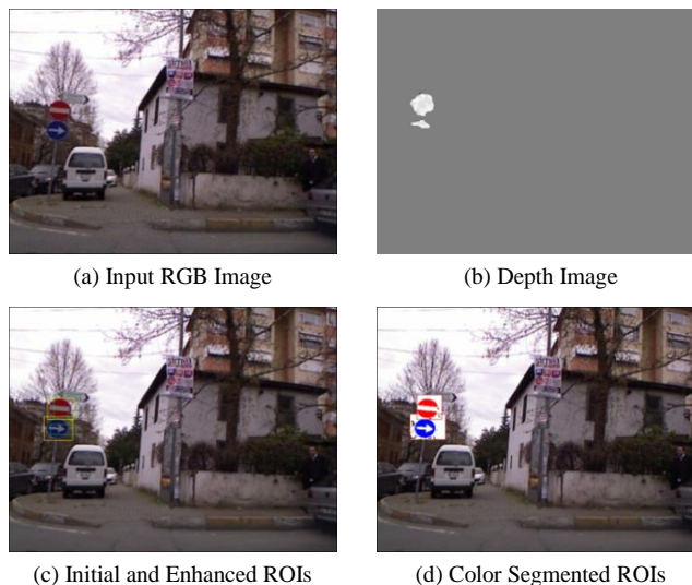
Figure 4 ROI detection with Kinect sensor
