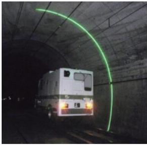
(a) A inspection vehicle for normal-speed railway tunnels
