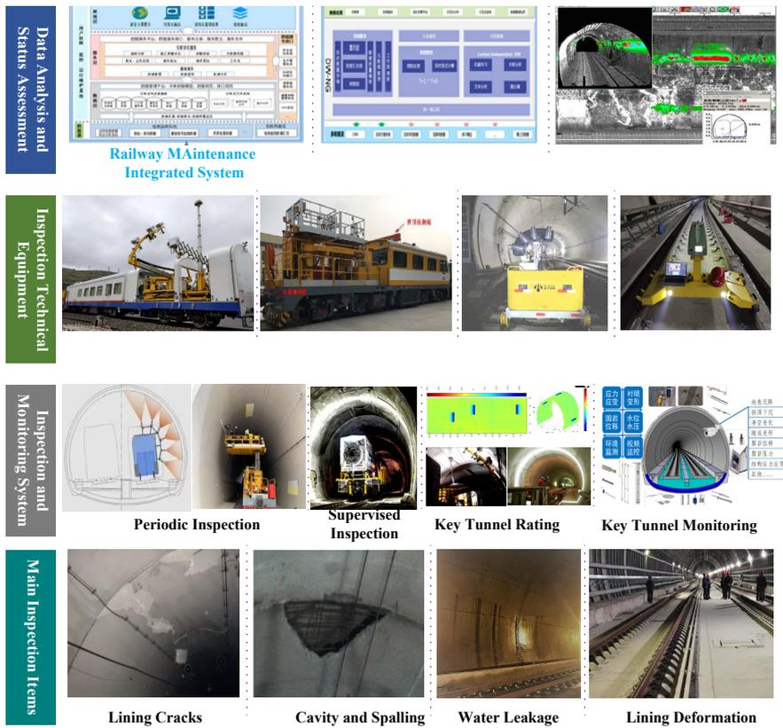
Figure 8 Framework of railway tunnel inspection system
